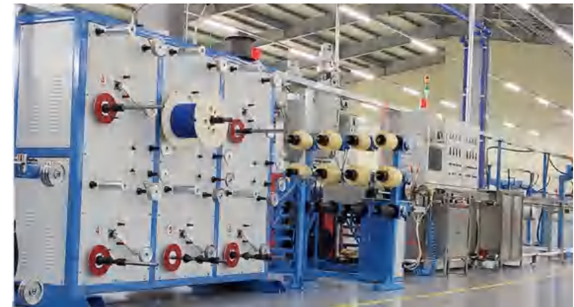
50mm FTTH皮线光缆+单双芯光缆挤出生产线 FTTH drop cable+simplex/duplex cable production line
