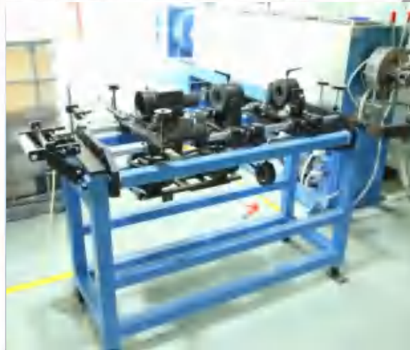
钢铝带成型装置 Steel-Aluminum tape longitudinal forming device
