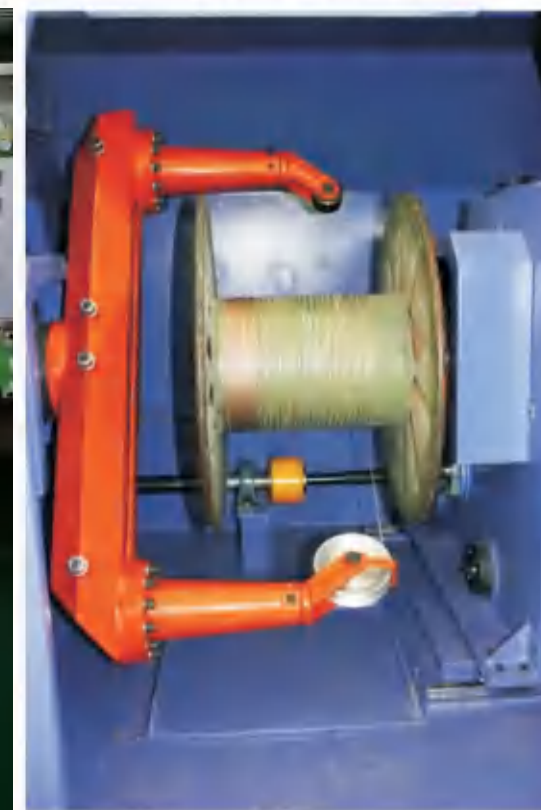
悬臂单绞机内部转体结构 Cantilever stranding machine inside structure
